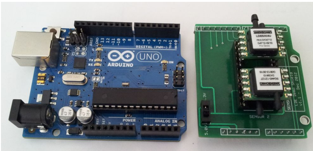
Figure 1: The Arduino Uno (left) and the LDE demo shield with two LDE sensors (right).
