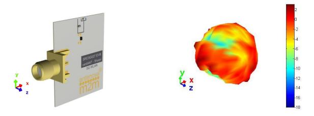
**3D pattern at 5.46GHz** Drag to rotate pattern and PCB by using Adobe Reader (Click to Activate)
