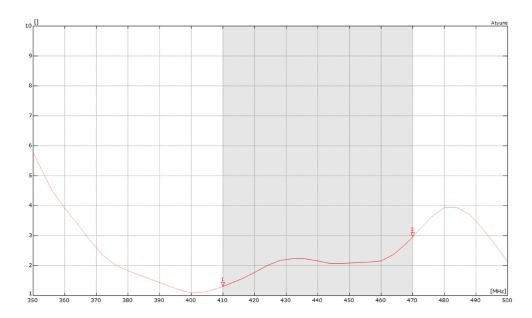
All data measured on SRFI079-150 in a loaded condition adhered to a plastic carrier in free space.
