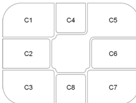
Figure 5. D18 micromodule contact assignment
