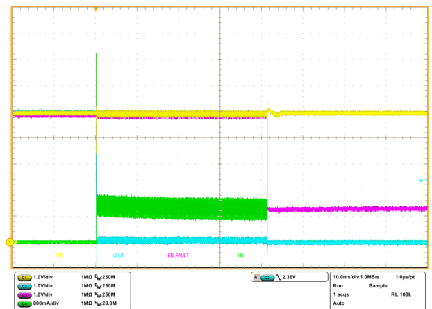
Figure 29. Output short-circuit during operation
