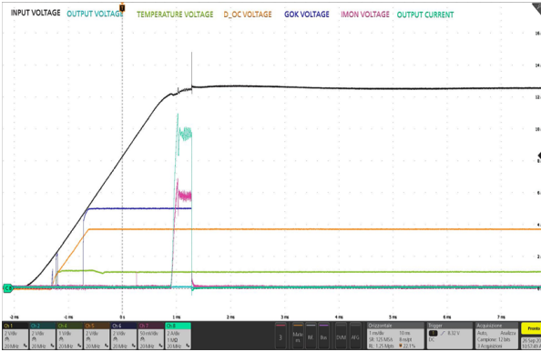
Figure 32. Startup into output short-circuit
