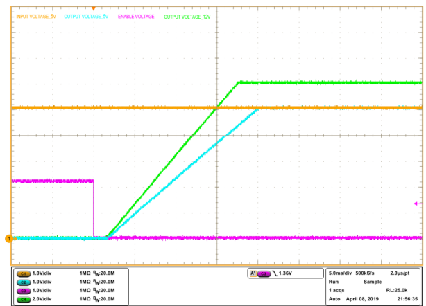
Figure 8. Start-up by EN, no load
