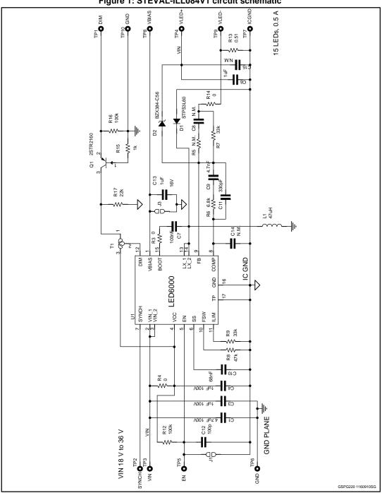
Figure 1: STEVAL-ILL084V1 circuit schematic
