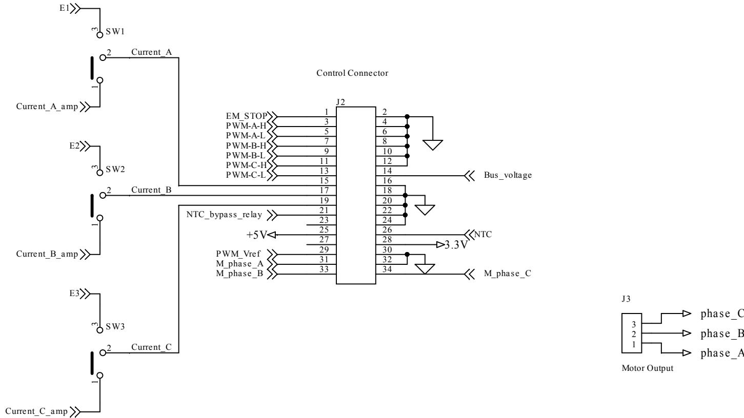
Figure 3. STEVAL-IPMNM5Q board schematic (3 of 5)
