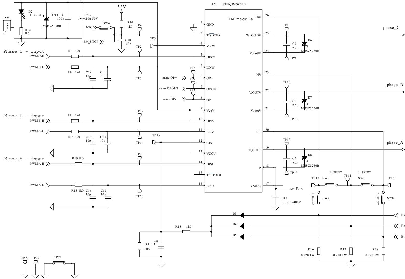
**Figure 5. STEVAL-IPMNM5Q board schematic (5 of 5)**
