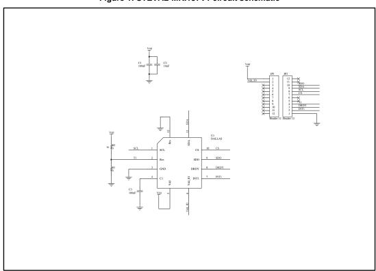
Figure 1: STEVAL-MKI137V1 circuit schematic
