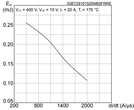
Figure 25. Reverse recovery energy vs diode current slope
