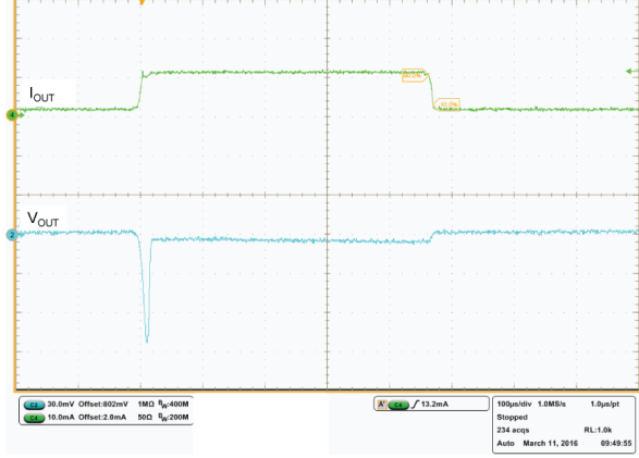
Figure 29. Load transient ( t_{rise} = 5 \mu s )
