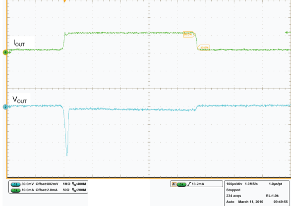
Figure 29. Load transient ( t_{rise} = 5 \mu s )
