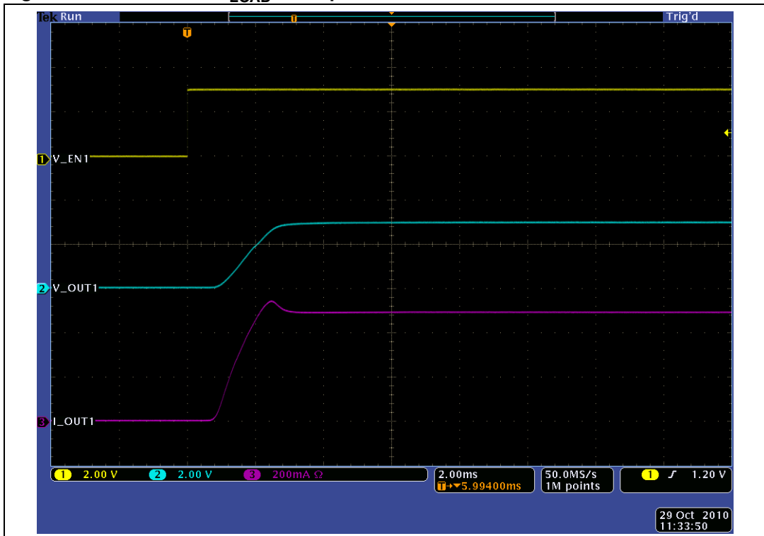
Figure 5. Turn-on for C_{LOAD} = 470 \mu F
