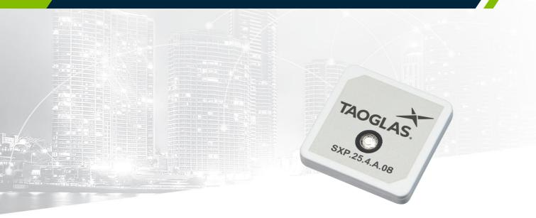
The Taoglas SXP.25.4.A.08 is part of a series of patch antennas designed for use with Satellite Digital Audio Radio Services (SDARS). It features left-hand circular polarization, low in-band axial ratio, and excellent gain characteristics in the 2320 to 2345 MHz band, making it compatible with the most popular satellite radio services available in many new vehicles.
