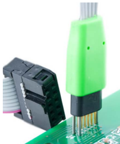
Figure 55 - Tag Connect Header inserted into PCB
