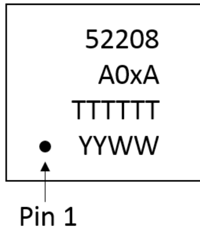
Figure 10.10. Si52208 Top Marking
