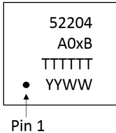
Figure 10.11. Si52204 Top Marking
