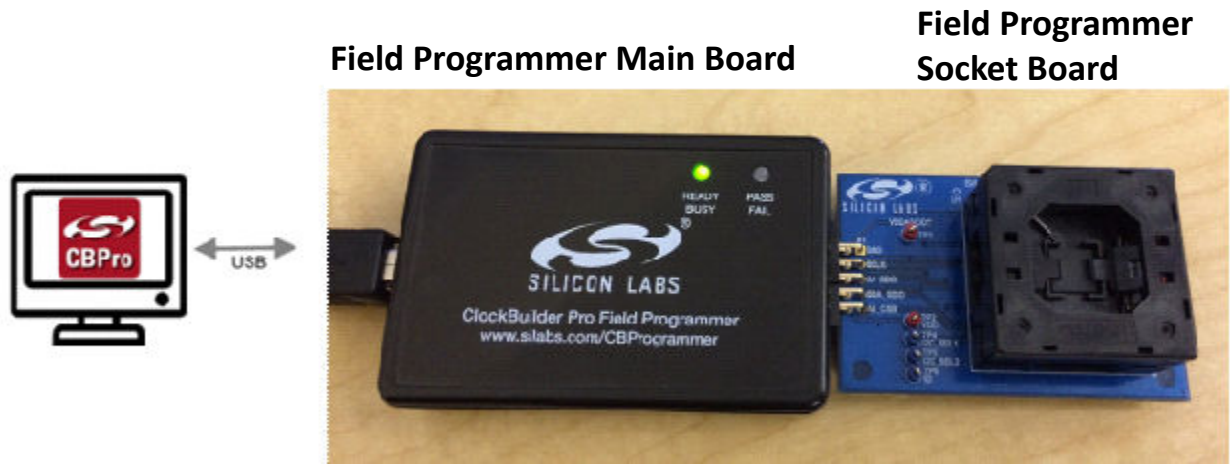
Figure 4.3. System from PC to Programming CBPROG-DONGLE Board to Field Programmer Socket Board
