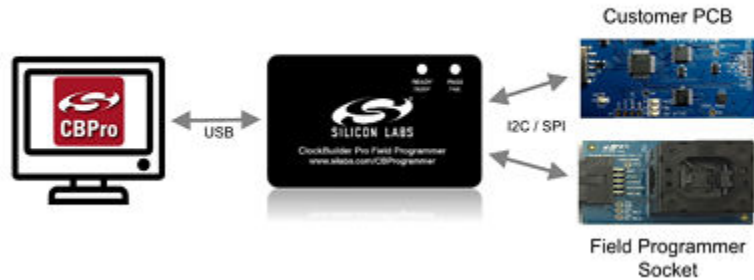
Figure 4.1. PC to CBPROG-DONGLE Connection
