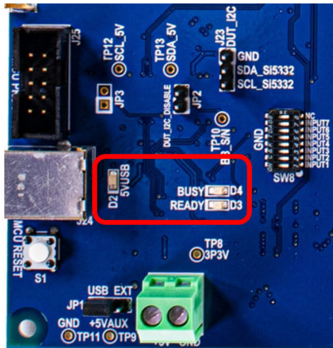
Figure 3.2. Si5332-8A-EVB LED Locations
