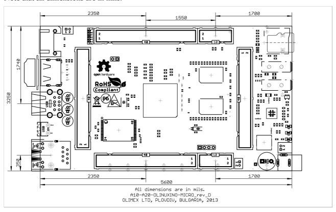
The three highest elements on the board in order from the tallest to the shortest are: USB\_HOST connector – 700mils, capacitors C202 – 650mils, the Ethernet connector – 600mils.
