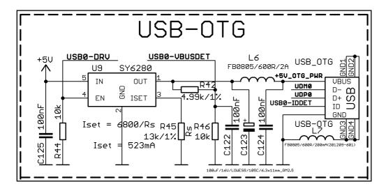
The USB\_OTG features Low Loss Power Distribution Switch SY6280 which protects the board in case the devices you have plugged to the USB\_OTG attempt to draw more current than 523mA combined. The maximum current available on the 5V USB\_OTG is exactly 523mA.
