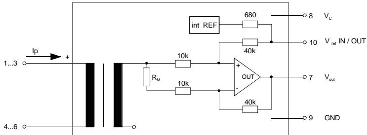
**Possibilities of wiring** (@ T<sub>A</sub> = 85°C)
