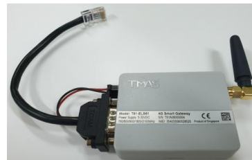
Cable connection to modem
