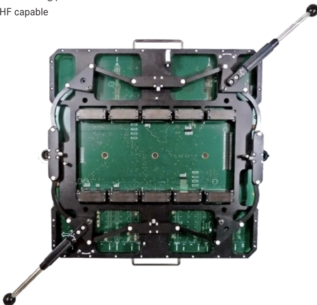
Universal Interface Board with Locking Mechanism, open position (no DUT)
