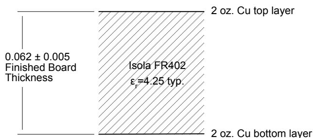
TriQuint Evaluation Board PCB Material and Stack-up
