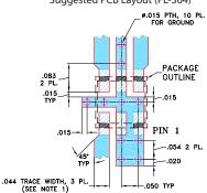
NOTES: 1. TRACE WIDTH IS SHOWN FOR ROGERS RO4350B WITH DIELECTRIC THICKNESS .020" ± .0015"; COPPER: 1/2 0Z. ON EACH SIDE. FOR OTHER MATERIALS TRACE WIDTH MAY NEED TO BE MODIFIED.
