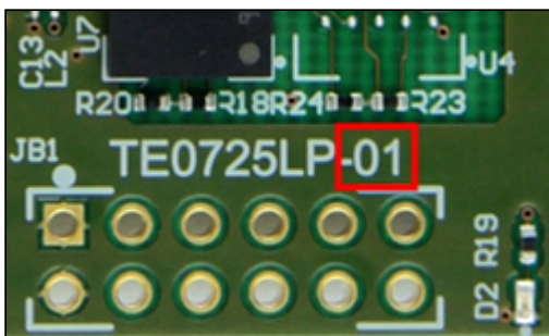
Figure 6: Module hardware revision number
