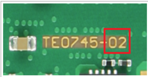
Figure 7: Board hardware revision number.
