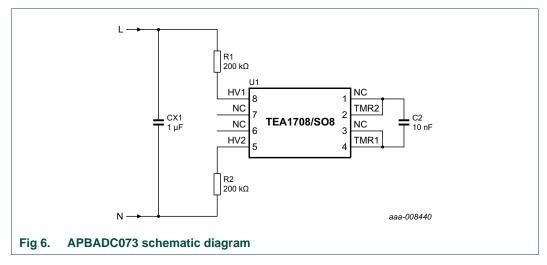
On the demo board, pin 1 (NC) and pin 2 (TMR2) are connected. Pin 3 (NC) and pin 4 (TMR1) are also connected. The reason for this is backward compatibility with earlier (test) versions of the TEA1708T.
