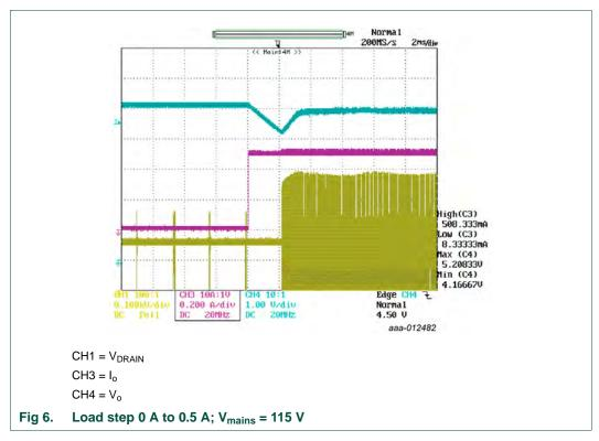
In the worst case (see Figure 6), the output voltage drops to 4.17 V which fulfills the USB-charger specification 1.1.
