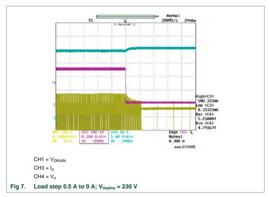
After the load step from 0.5 A to 0 A, the output voltage rises from 4.8 V to 5.25 V.
