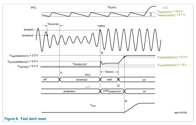
Before t1, the LLC (and/or PFC) is in a (latched) protection and pulls down the SNSBOOST pin, which also disables the PFC.
