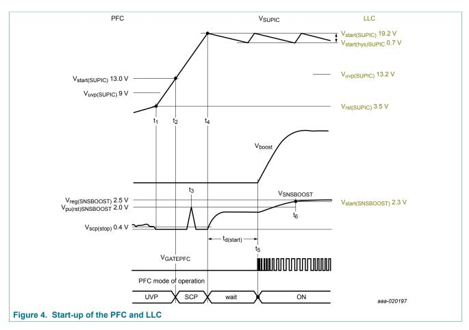
The exact start-up sequence of the PFC depends on the availability of start-up conditions (brownin level,  $V_{\text{start}(SUPIC)}$  of the PFC, and  $I_{\text{en}(PFC)}$ ).
