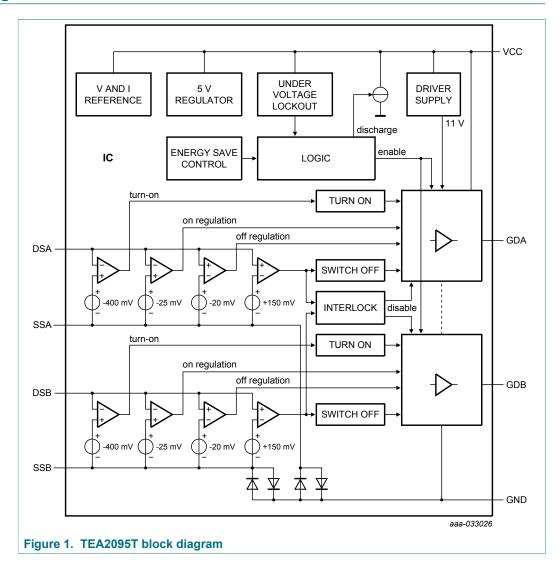
GreenChip dual synchronous rectifier controller
