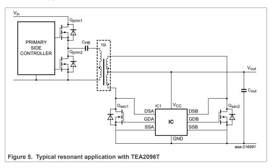
GreenChip dual synchronous rectifier controller
