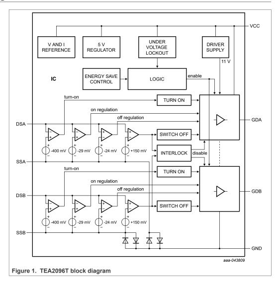
GreenChip dual synchronous rectifier controller
