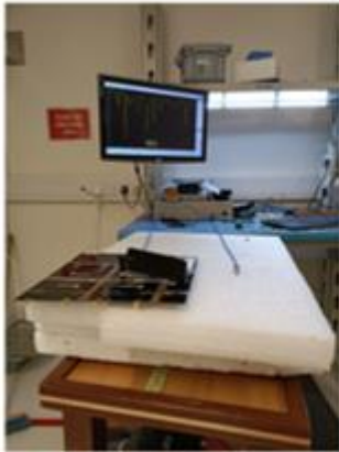
Chamber & VNA setup bent in the middle of a 30x30cm ground plane
