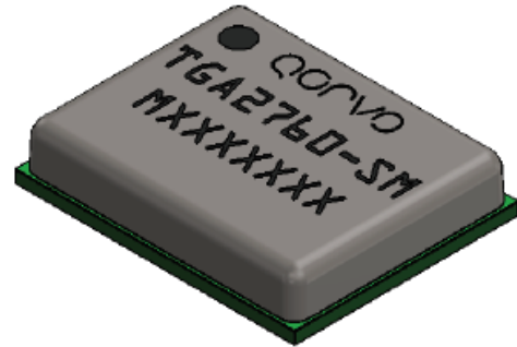
20-Lead 8.0 x 10.0 x 2 mm Package
