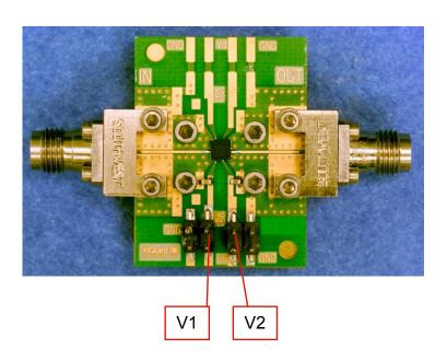
GaAs MMIC devices are susceptible to damage from Electrostatic Discharge. Proper precautions should be observed during handling, assembly and test.
