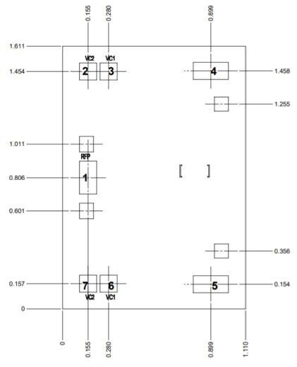
Unit: millimeters Thickness: 0.10
