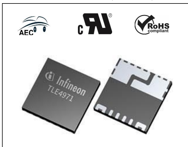
Coreless current sensor in PG-TISON-8 package
