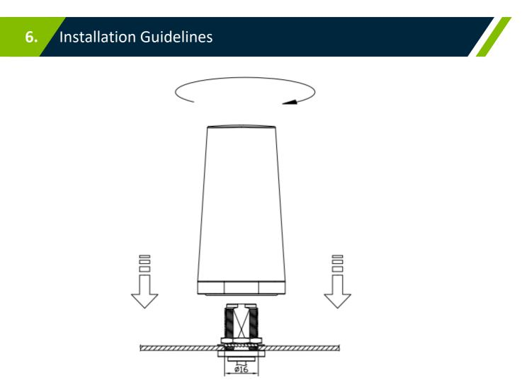
Recommended torque for mounting is 4.018 N.m or 41 kgf.cm Maximum torque for mounting is 9.8 N.m or 100 kgf.cm
