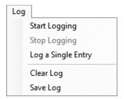
Click **Start Logging** to start the logging function. Each time the program polls the Prox information from the device, it will create a new log entry showing the raw data values, the values of various control registers, and the values entered by the user into the text fields near the bottom right corner of the window.
