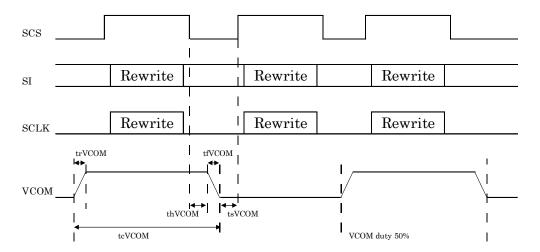
AC drive between 0 V and 3.3~V is required for VCOM signal.
