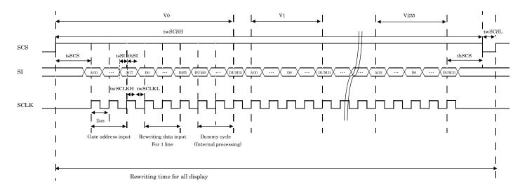
3 lines (SCS, SCLK, and SI) are control signals to rewrite.
