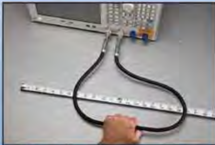
Cable is pulled off center 10" in both directions A brand new cable can have a break-in period of several hundred flexes
