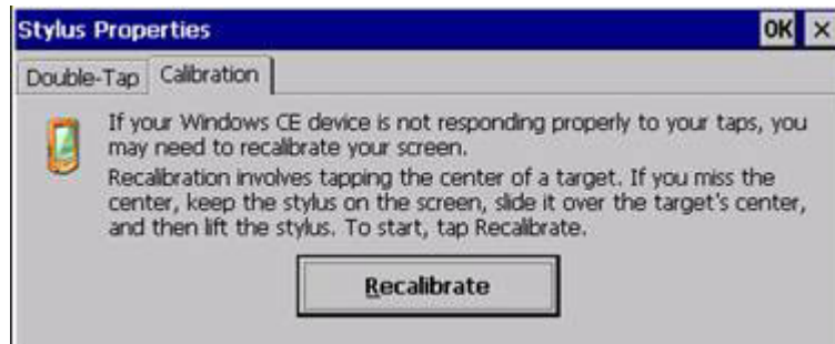
Figure 5.12 Touch panel calibration
