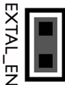
Figure 6-22: External Crystal Circuitry Enable (CT5)
