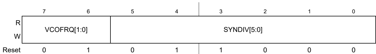
Figure 10-4. S12CPMU Synthesizer Register (CPMUSYNR)
