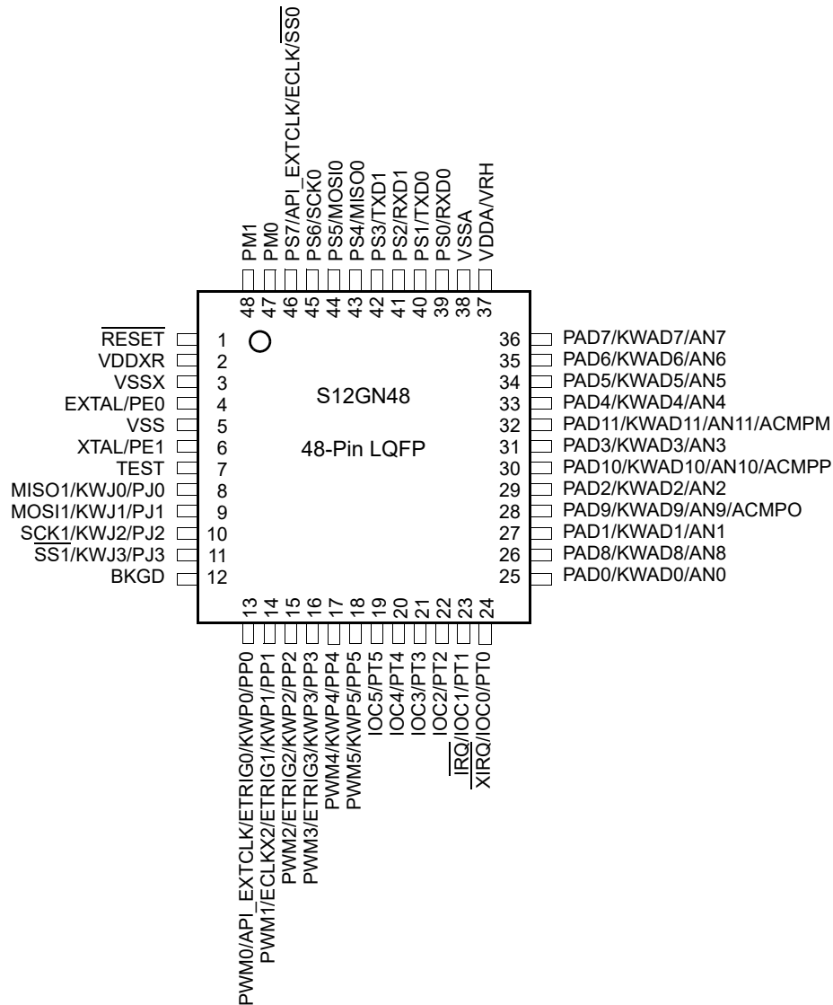
Figure 1-8. 48-Pin LQFP Pinout for S12GN48
