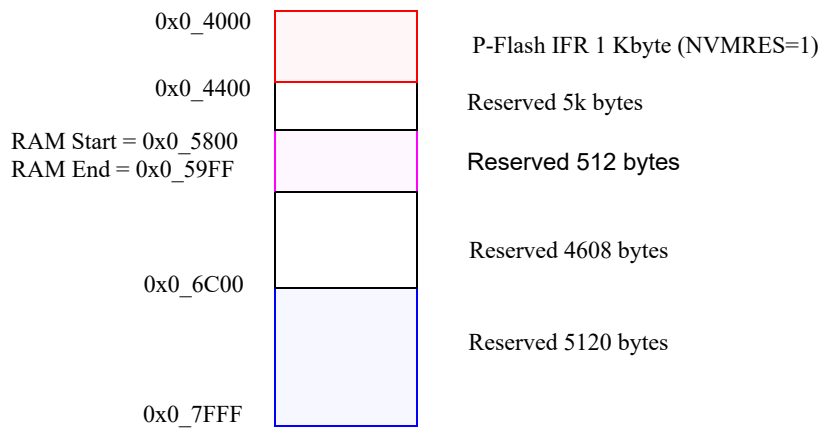
Figure 28-3. Memory Controller Resource Memory Map (NVMRES=1)
