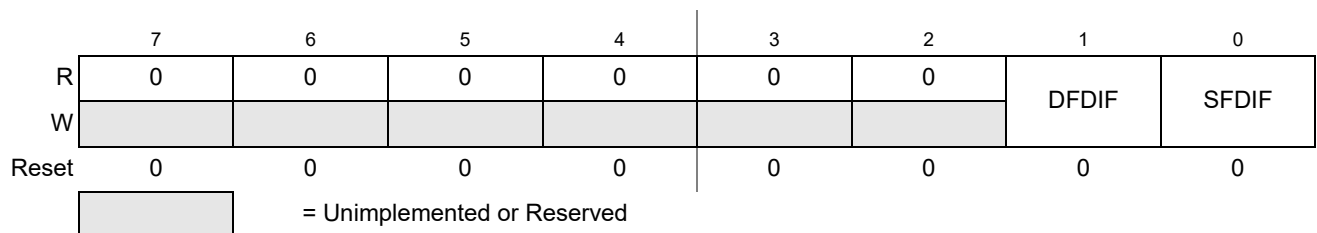
Figure 27-12. Flash Error Status Register (FERSTAT)
