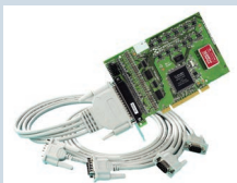
UC-368: uPCI 4xRS422/485 1MBaud Opto Isolated
