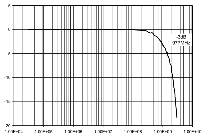
Typical Insertion Loss (S21) 30KHz to 3GHz
