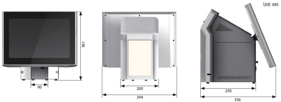
Figure 1.1 Dimensions of UPOS-3150
