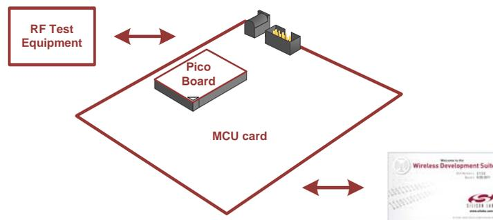
Using the WDS Chip Configurator software is the best way to evaluate the RF performance in the lab with a PC in various configurations. The WDS GUI provides a convenient way to run configuration scripts and to change the radio settings bit-by-bit.
