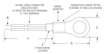
Dim "L" is the MIN lead wire length, and is specified by the last two digits of the part number (USUR1000-xxx-xx) e.g. USUR1000-102G-03 would have a MIN lead wire length of 3"
