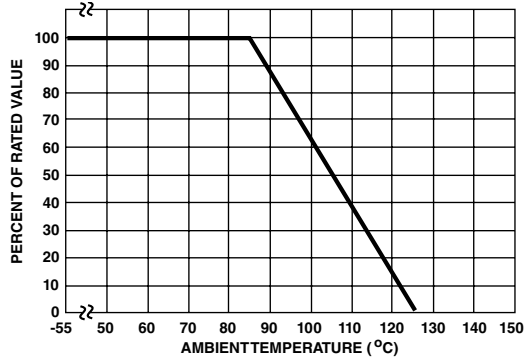
1A - Power Derating for Epoxy Coated
